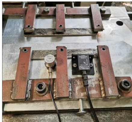
Figure 1 Fixtures, weldments and sensors for vibration measurement
