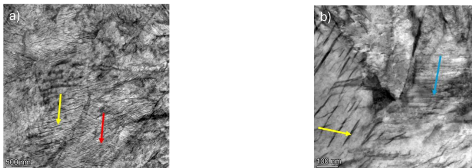
Figure 2 TEM BF micrographs of BQT 350 sample, a) the locality with transition carbides which replaced the original twinning population and b) neighbouring areas with remaining twins and with transition carbides. Yellow arrows show the transition carbides, blue arrows show the population of short twins. The red arrow designates the area with both transition carbides and rests of twins.
