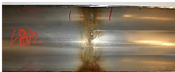
Figure 4 Corrosion of cross welds in a pipe in branch B
