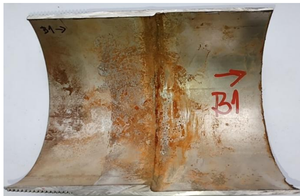
Figure 3 Corrosion attack of cross welds, fillet weld of nozzles and inner surface of a pipe in branch A
