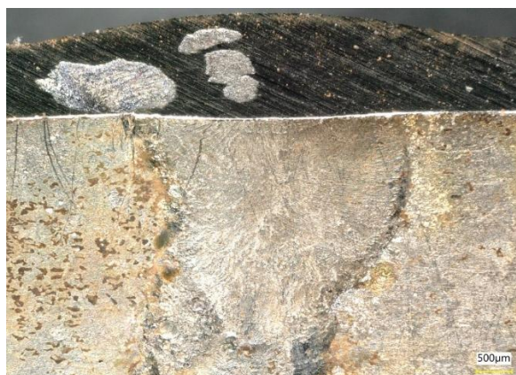
Figure 6 Corrosion pits inside the weld metal, pipe in branch B
