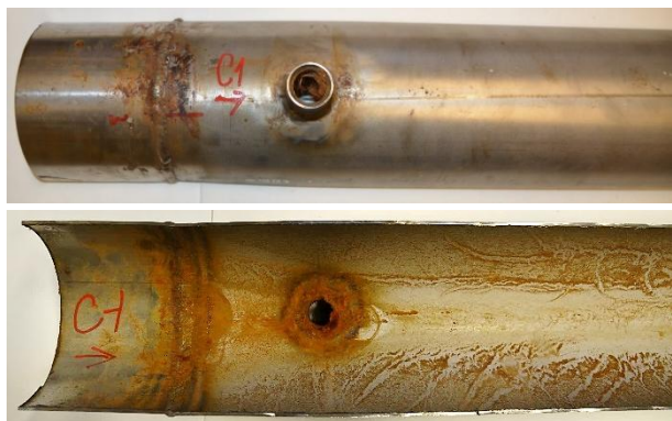
Figure 3 Corrosion attack of cross welds, fillet weld of nozzles and inner surface of a pipe in branch A
