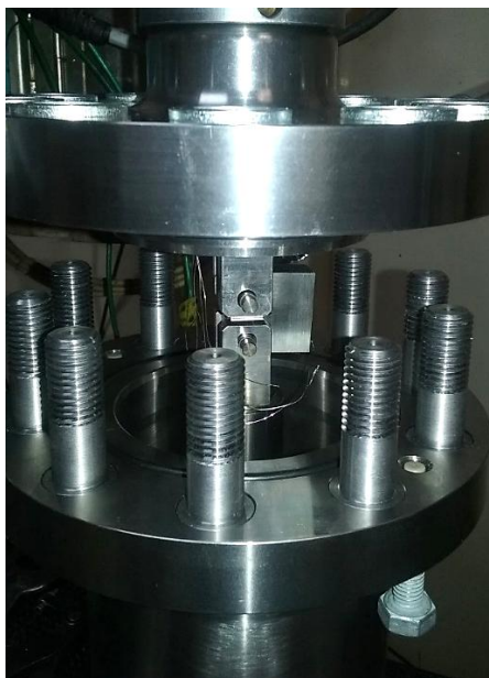
Figure 1 Autoclave built-in testing machine, CT specimen in jaws
