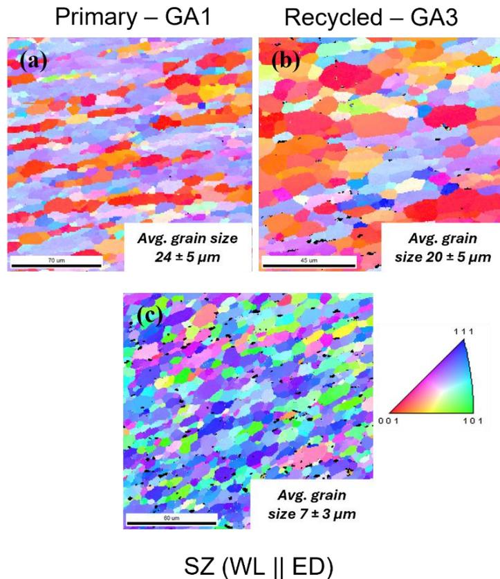
**Figure 4** Variation in recrystallized grain size between the BMs (a & b) and the SZ (c) in the WL || ED weld
