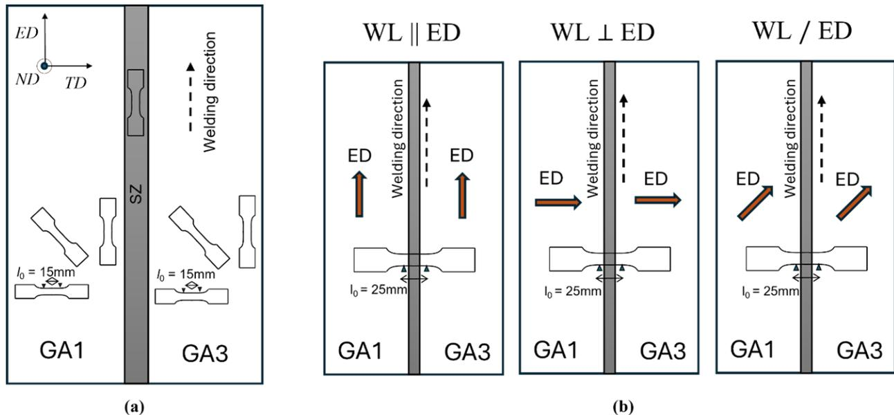
**Figure 2** Sample extraction plan for the tensile studies: (a) Orientations of the tensile specimens extracted from BMs and SZ, (b) Location of the transverse tensile specimens extracted from TWBs with respect to the different weld line orientations
