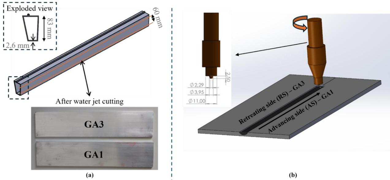
**Figure 1** Outline of the experimental setup used in the FSW trials: (a) Sheet preparation, (b) Tool design and welding conditions
