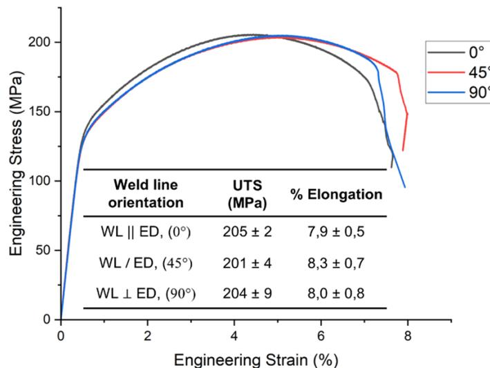
**Figure 6** Transverse tensile properties of TWBs for different weld line orientations
