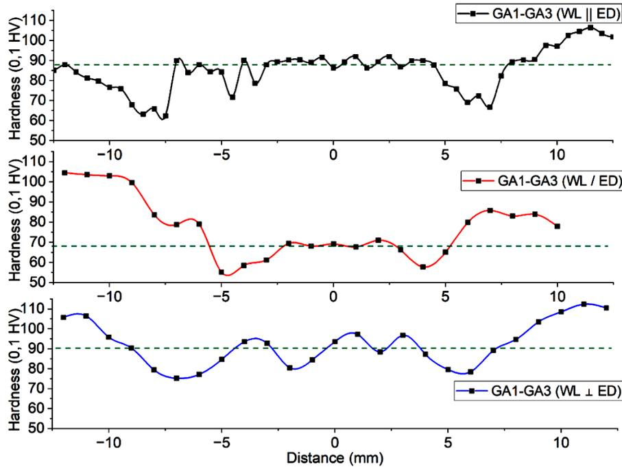
**Figure 5** Hardness profile for TWBs in different weld line orientations
