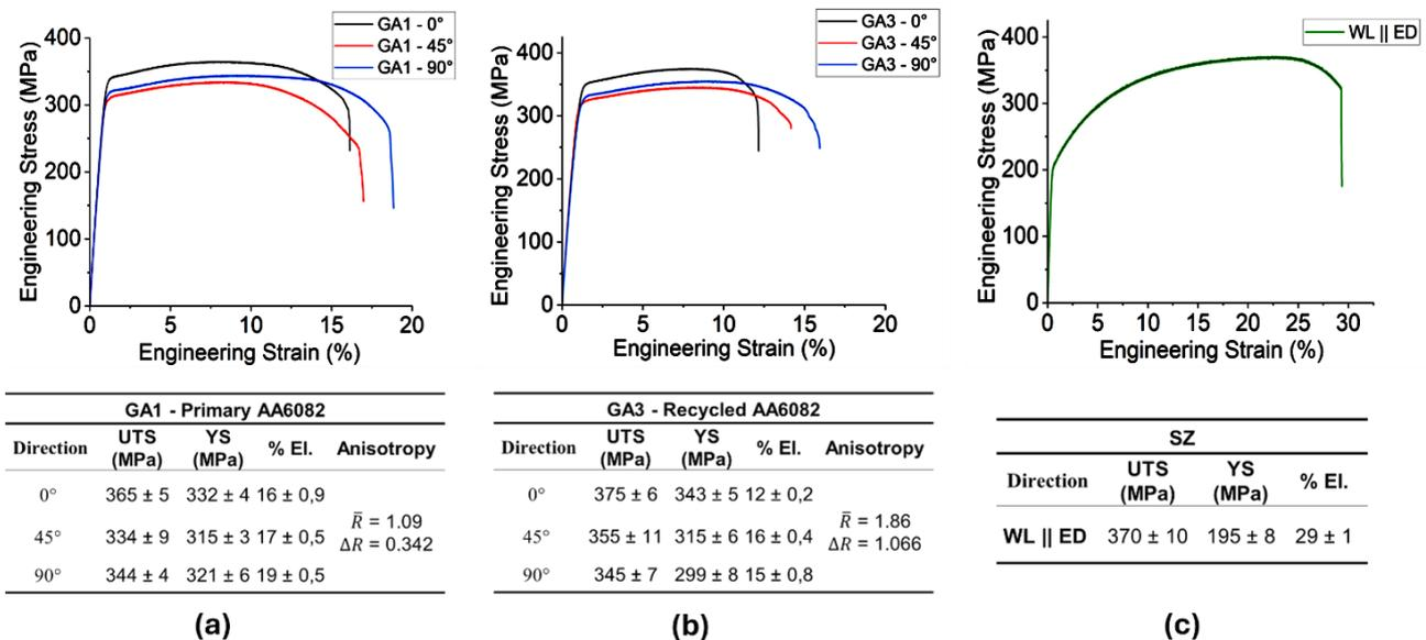
**Figure 3** Compilation of different engineering stress-strain curves; (a) GA1 - Primary AA6082, (b) GA3 - Recycled AA6082 & (c) SZ – extracted from the WL || ED weld
