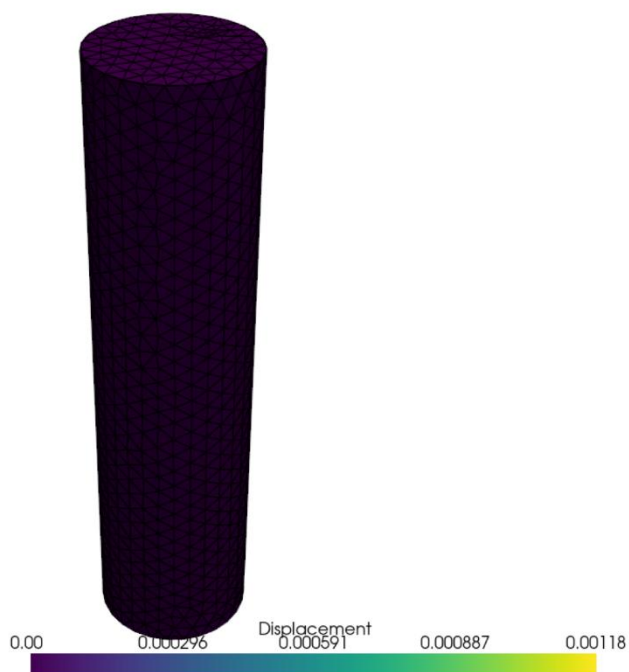
Figure 2 Structural displacement distribution (0 to 1.182415 mm)
