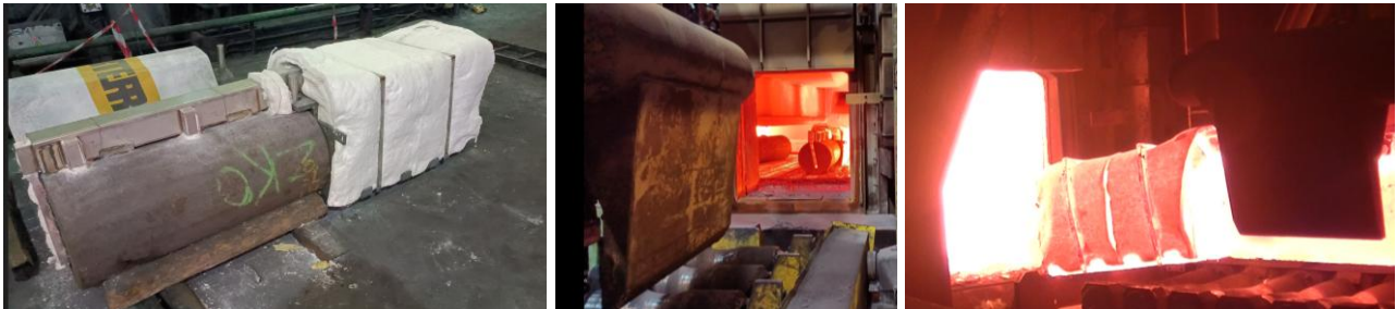
Figure 2 Bloom with embedded sensors and connected insulated box with data logger (left); cold bloom inserted into furnace (center) and hot bloom removed from furnace (right)
