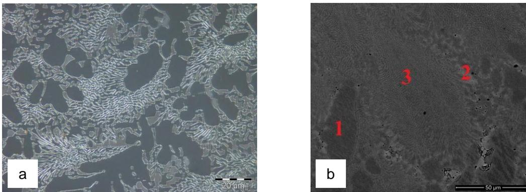
**Figure 3** Microstructures of in-situ composite FeSi-NiAl (2:1), a) LOM, b) SEM
