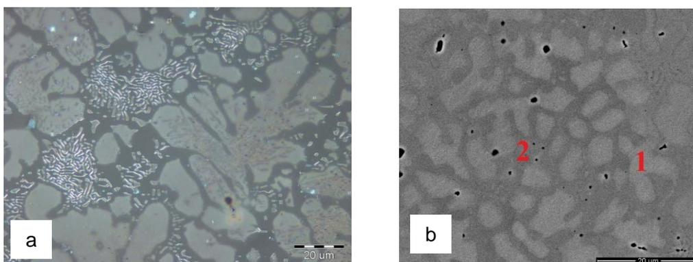
**Figure 2** Microstructures of in-situ composite FeSi-NiAl (1:1) after heat treatment, a) LOM, b) SEM
