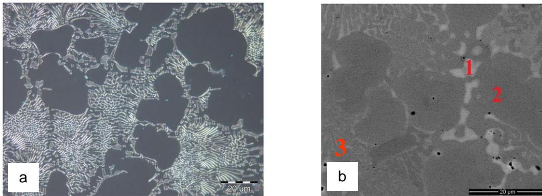
**Figure 4** Microstructures of in-situ composite FeSi-NiAl (2:1) after heat treatment, a) LOM, b) SEM
