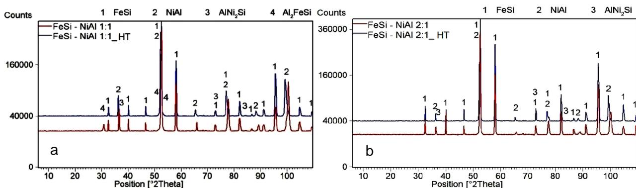
**Figure 5** Diffraction record for samples (a) FeSi-NiAl 1:1 (as-cast) and (b) FeSi-NiAl 1:1 TZ (after heat treatment)
