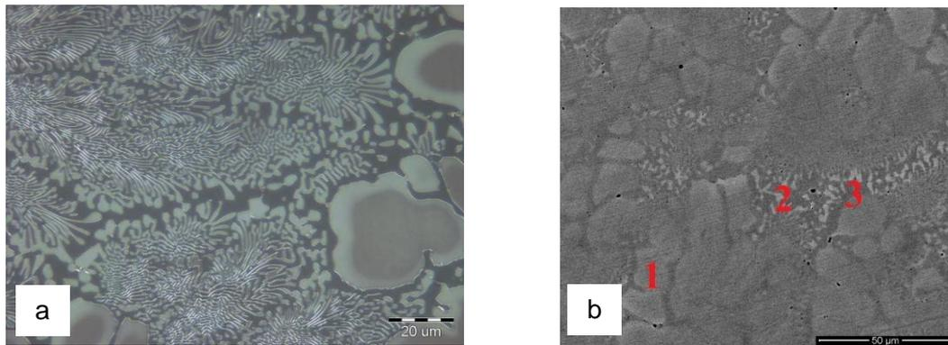
**Figure 1** Microstructures of in-situ composite FeSi-NiAl (1:1) in as-cast state: a) LOM, b) SEM
