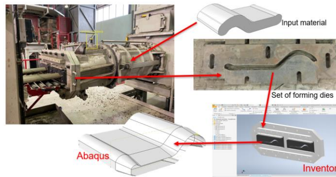
Figure 5 Preparation of a numerical model for the extrusion of a clay band assigned for ceramic roof tiles
