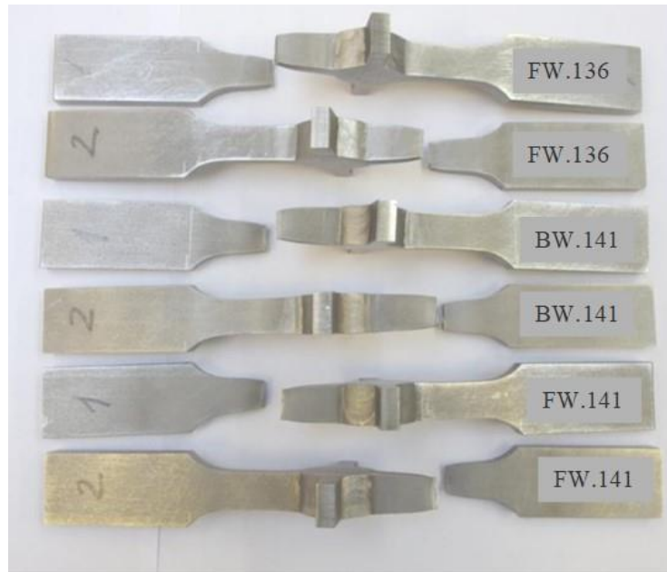
Figure 3 The view of x-type specimens after the static tension experiment
