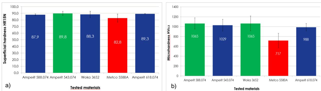
**Figure 2** Graphs of basic mechanical properties: a) superficial hardness HR15N, b) microhardness HV0.3
