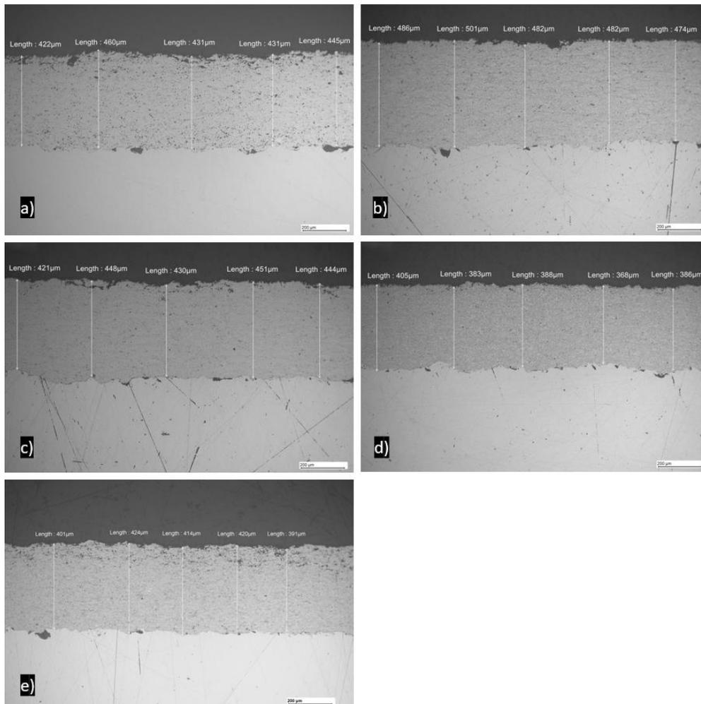
**Figure 1** Microstructures of the tested coatings at 100x magnification: a) Amperit 588.074, b) Amperit 543.074, c) Woka 3652, d) Metco 5580A, e) Amperit 618.074
