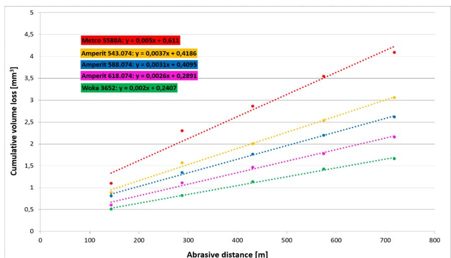
**Figure 3** Cumulative volume loss of material depending on the traveled path after the abrasive wear resistance test.
