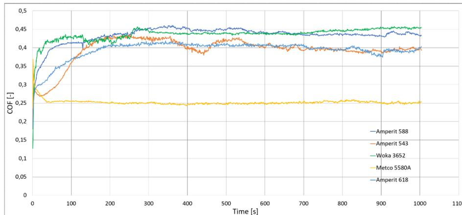
**Figure 4** The course of the COF as a function of time for all tested materials
