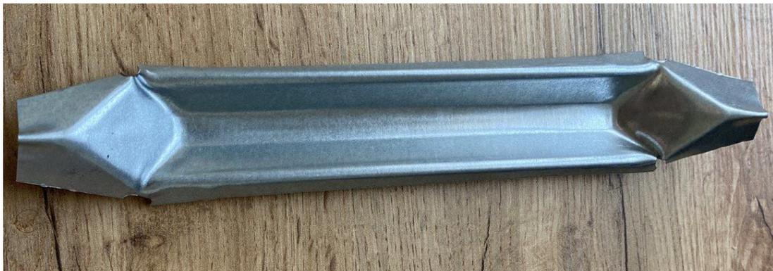
**Figure 8** Pressed part of the lock cover
