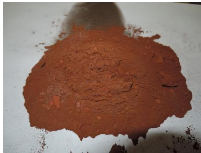
Figure 8 Effect of temperature on the colour change of steelmaking sludge (SNG), processed in a nitrogen atmosphere with graphite at 800 °C
