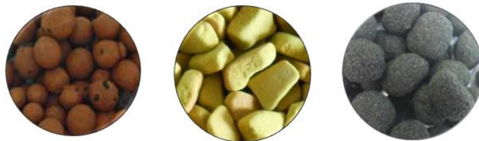
Figure 3 Example of individual types of precursors, from left ceramic material based on Al_2O_3 \cdot SiO_2 , shards of cores (Croning technology), furan no-bake mixture [18]
