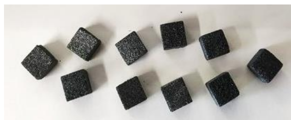
Figure 7 Shape of precursors after removal from the core box
