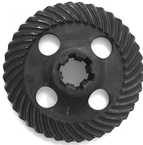
Figure 3 One element of spiroid gears: face gear in real
