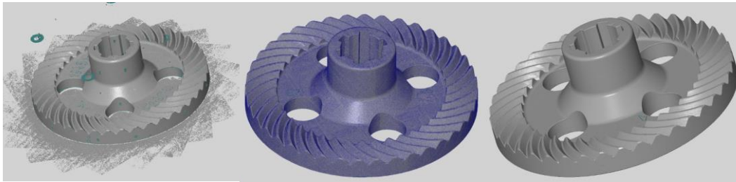
Figure 5 Raw data of point cloud (left), polygonized surface of the measurement object with the polygons displayed (middle), and the object after polygonization (right)
