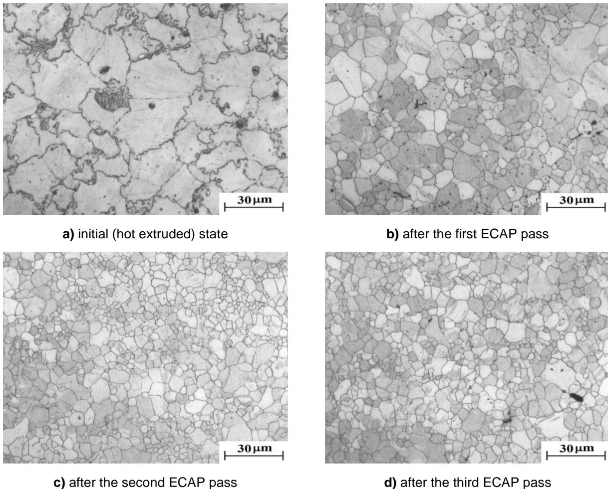
**Figure 2** The OM images of the microstructure of AZ61
