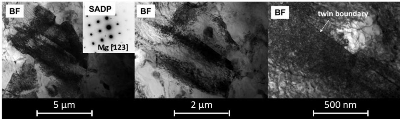
**Figure 3** Set of bright field (BF) images and corresponding selected area diffraction pattern (SADP) of sample after 1 pass of ECAP
