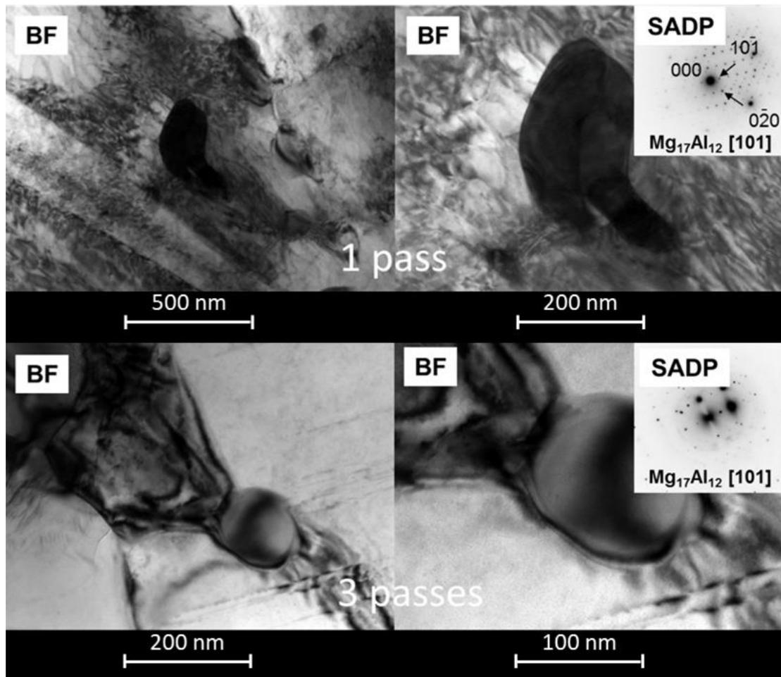
**Figure 5** BF images taken at different magnifications and corresponding SADPs of samples after 1 (upper) and 3 (lower) passes, respectively
