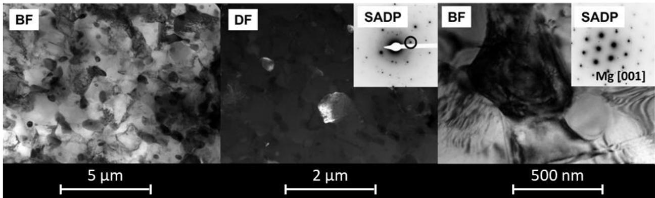
**Figure 4** Set of bright field (BF) images and corresponding selected area diffraction pattern (SADP) of sample after 3 pass of ECAP
