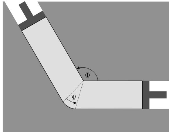
**Figure 1** Schematic illustration of ECAP die geometry [14]
