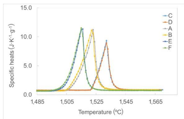
**Figure 5** Experimental values of specific heats of alloys A, B, C, D, E and F in the temperature range 1,485 – 1,580 °C
