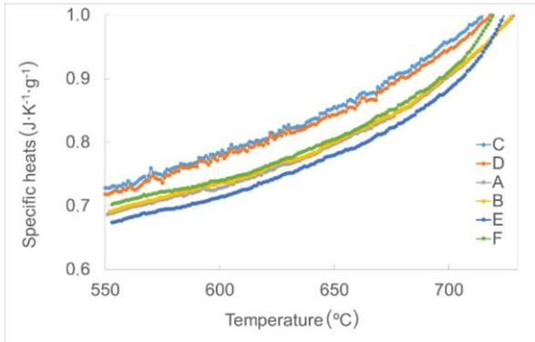
**Figure 2** Experimental values of specific heats of alloys A, B, C, D, E and F in the temperature range 550 - 730 °C
