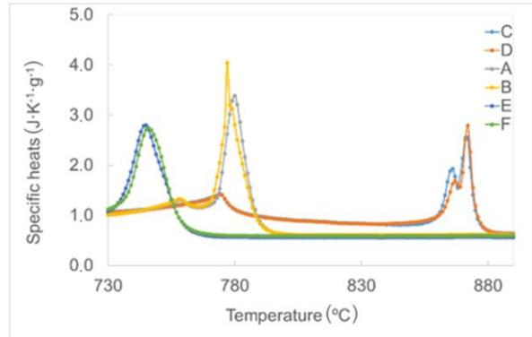
**Figure 3** Experimental values of specific heats of alloys A, B, C, D, E and F in the temperature range 730 - 890 °C
