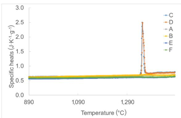
**Figure 4** Experimental values of specific heats of alloys A, B, C, D, E and F in the temperature range 890 – 1,485 °C
