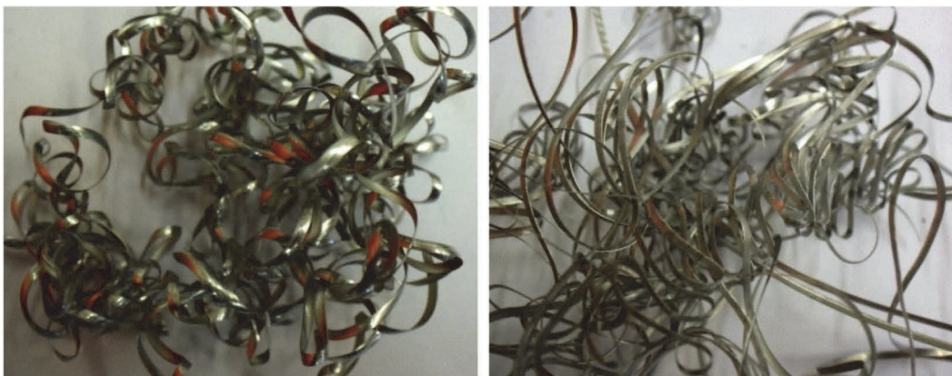
Figure 5 Chip forming r_n = 0-5 \mu\text{m} and r_n = 20-25 \mu\text{m}
