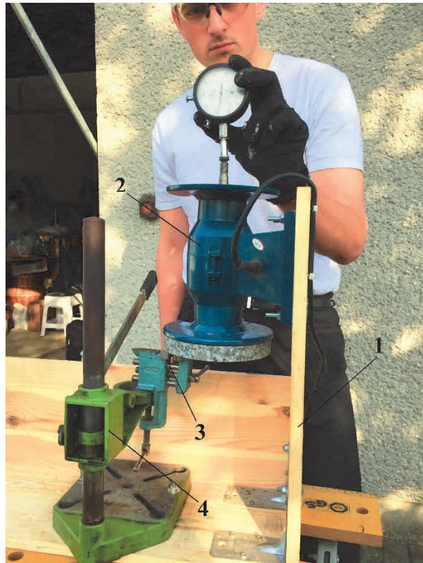
Figure 1 Author's stand for tribological tests of individual diamond segments
