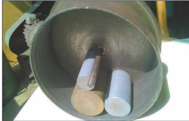
Figure 4 Interior view of the laboratory drum of the impact mill
