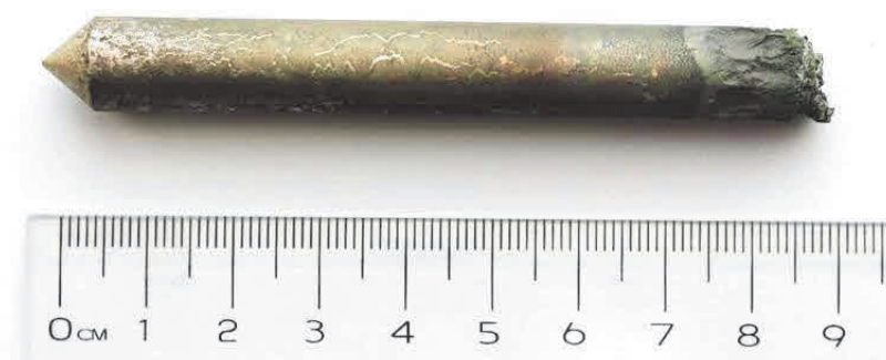
Figure 1 Sample of Ni-Al-Zr alloy in directed state
