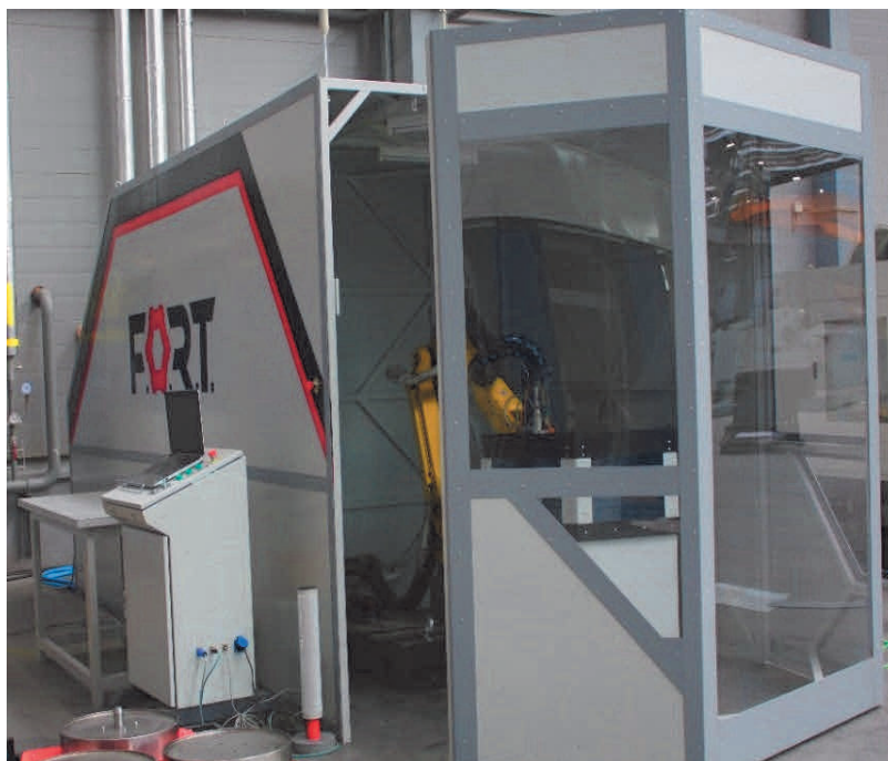
Figure 1 Additive installation of laser cladding
