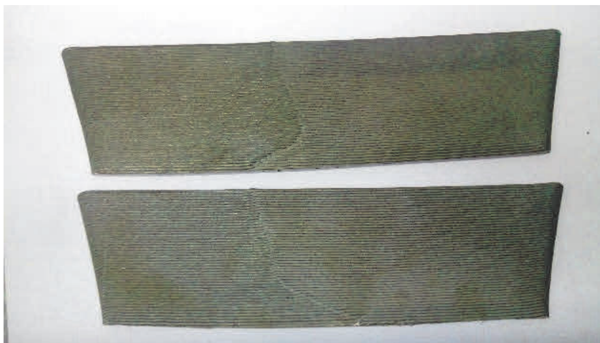
Figure 6 Single-pass walls of the Inconel 625 alloy
