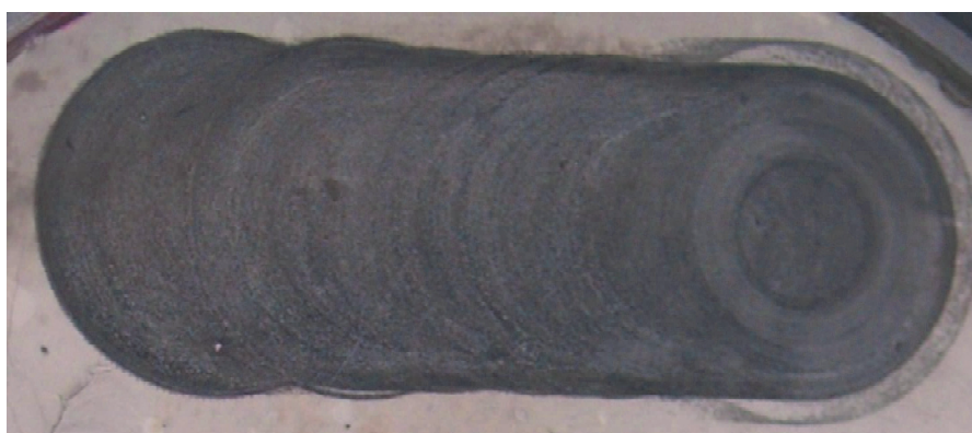
Figure 8 Titanium coating made with the following parameters: 6000 rpm; 50 N; 0.01 mm/min (own case study)
