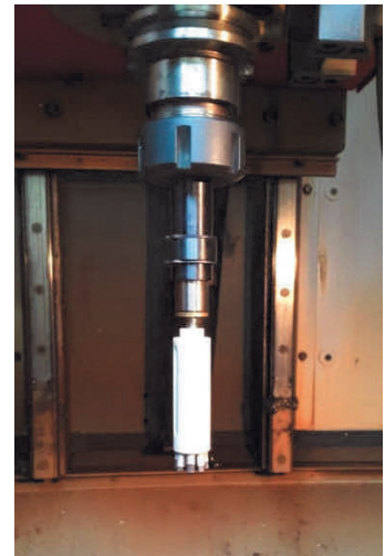
Figure 2 Prototype 1 tool with compensating handle mounted in the CNC machine spindle (own case study)
