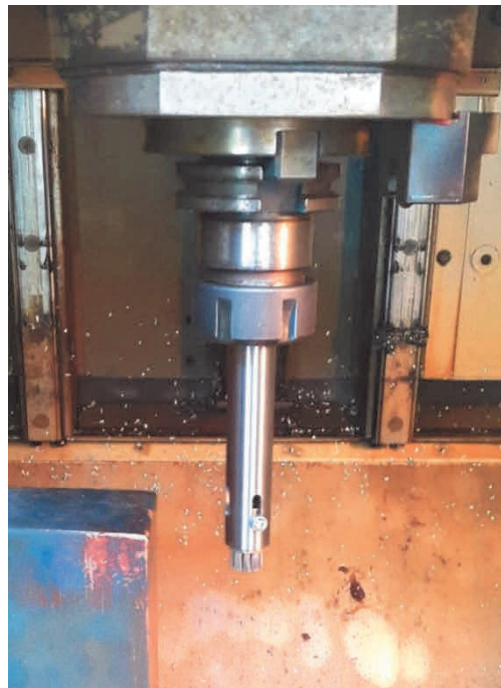
Figure 3 Prototype 2 tool with compensating handle mounted in the CNC machine spindle (own case study)
