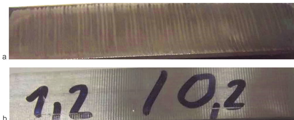
Figure 3 The example of cut edges - laser cut (a) and grinded (b)
