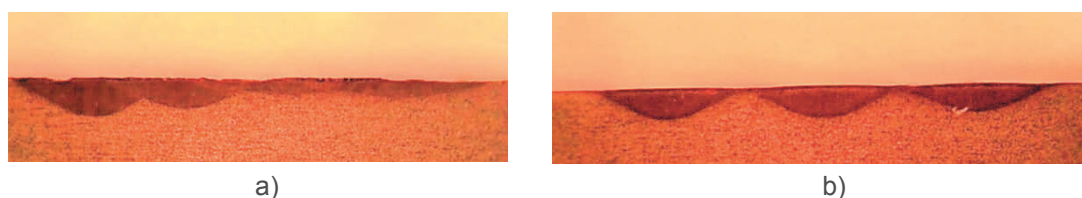
Figure 1 Macrosections of the treated samples: a) with 2.0 mm shift; b) with 3.0 mm shift
