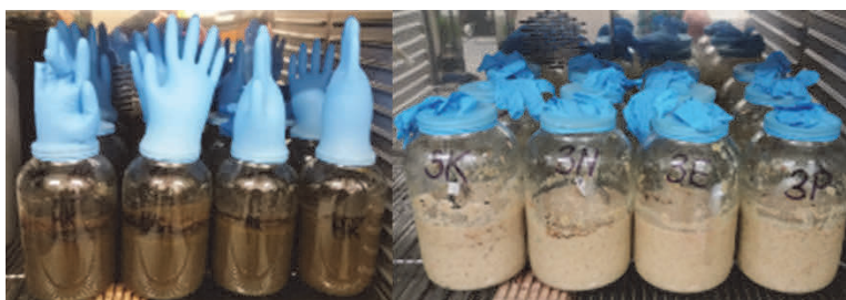
Figure 1 Sample incubation scheme Figure 2 Ring samples incubation in the 1 st and 2 nd corrosive media
