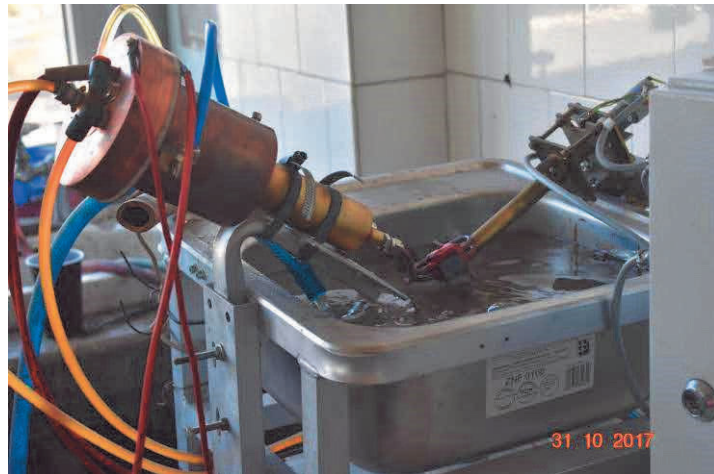
Figure 1 A device used during tests of thermal shock [6]
