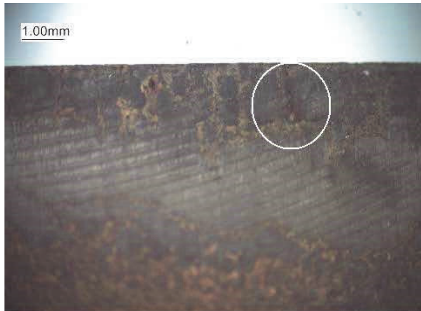
Figure 7 Macroscopic view of the sample surface after 4 series heat shock, marked crack of material
