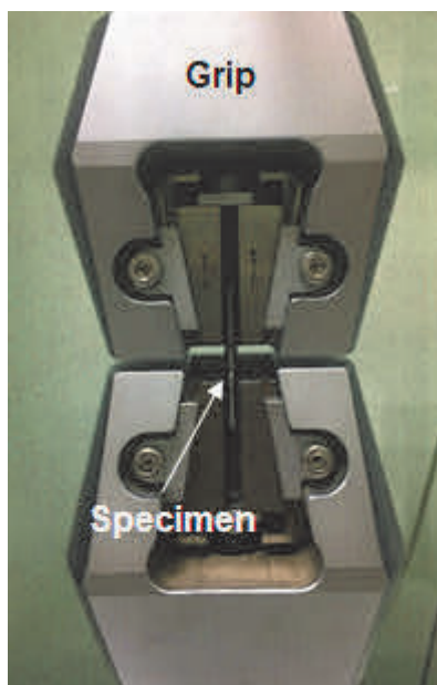
Figure 3 Mounting of tensile specimen with gripper before testing operates
