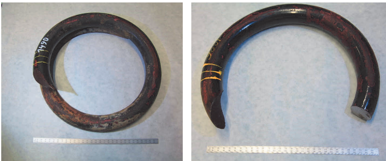
Figure 1 Fractured helical springs. (a) No. 1490 and (b) No. 1286
