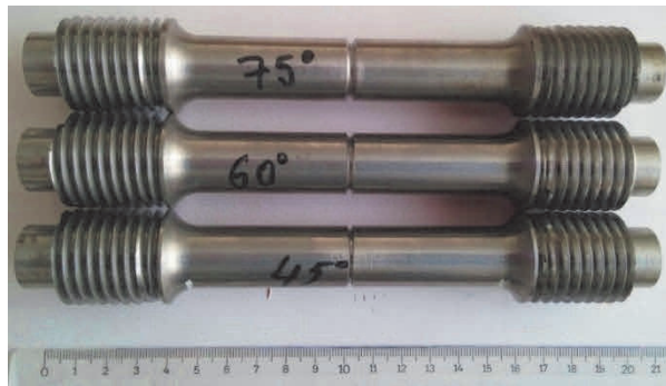
Figure 3 Notched specimens for fracture toughness testing
