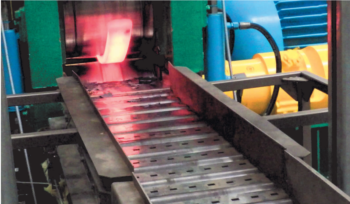
Figure 3 Example of rolling with critical asymmetry
