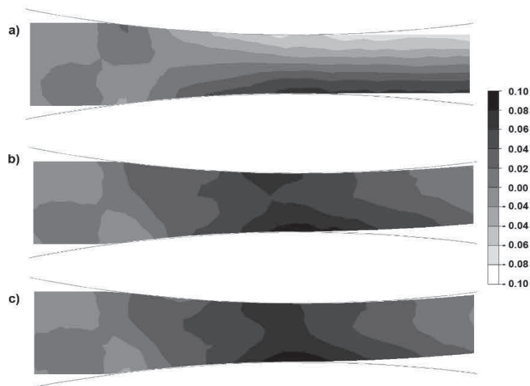
Figure 3 Distribution of the shear strain ( \varepsilon_{12} ) for analyzed cases of rolling: a) a_v = 1.0 , b) a_v = 1.3 , c) a_v = 1.5
