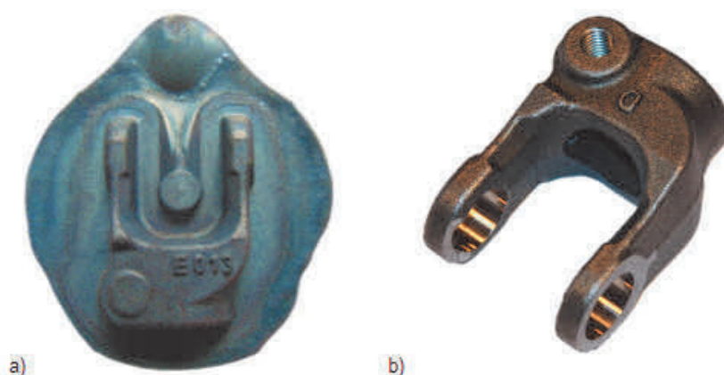
Figure 2 a) yoke type forging with flash, b) ready to use part after mechanical processing
