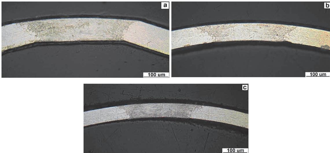
**Figure 5** The weld joint of tube THYSEN after a) welding, b) the first draw, c) the second draw
