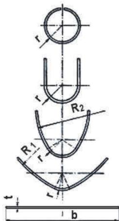
**Figure 1** Technological process of seam tubes production by bending proces
