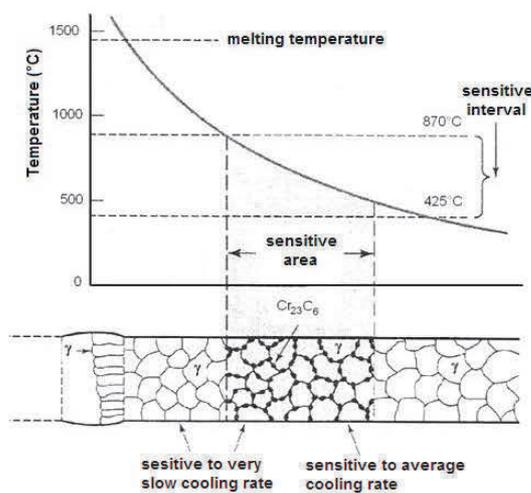
**Figure 6** The effect of temperature on Cr-Ni austenitic stainless steel microstructure in HAZ (left) [8]
