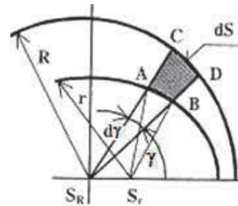
**Figure 11** The elementary surface on cross section of eccentric tube [4]
