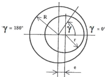
**Figure 10** The tube eccentricity [4]
