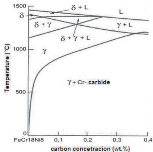
**Figure 7** The pseudo binary diagram of Fe18Cr8Ni and carbon (right) [8]
