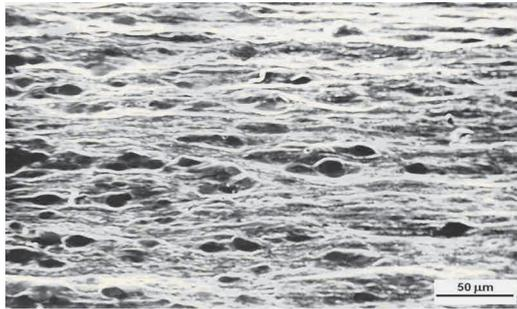
**Figure 8** The tube inner surface of material WESTIG 0.65 mm
