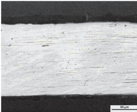
**Figure 3** The tube WESTIG longitudinal section
