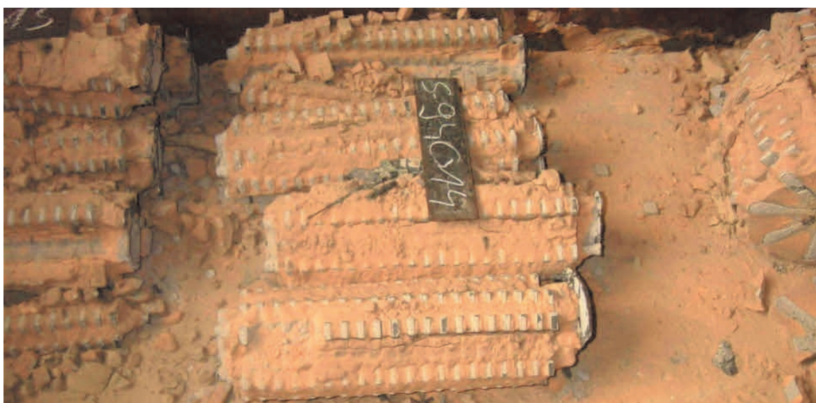
Figure 4 The Alnico 400 magnets after removing from the moulding flasks
