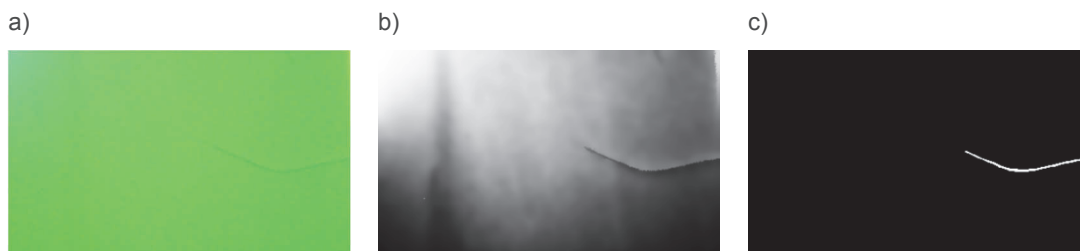
Figure 6 Fragment of blade image with a crack (a), denoised image with edge enhancement (b), and crack detected with Sobel and binarization filter (c)
