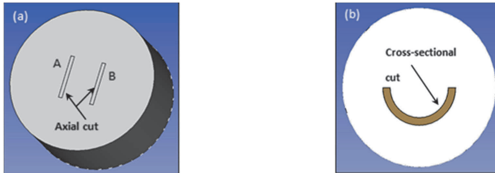
Figure 2 Sectioned sample embedding in an epoxy resin (a) in the axial / longitudinal direction, (b) in transverse direction
