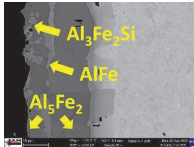
Figure 7 AS150 coating after heating at 885 °C
