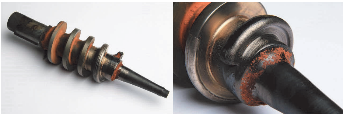
Figure 5 The laser cladded milling screw after testing in production
