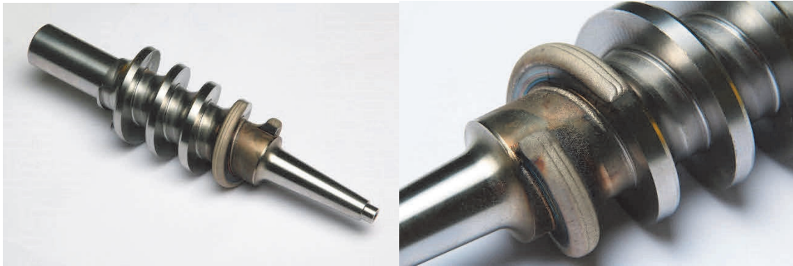
Figure 4 The milling screw after laser cladding
