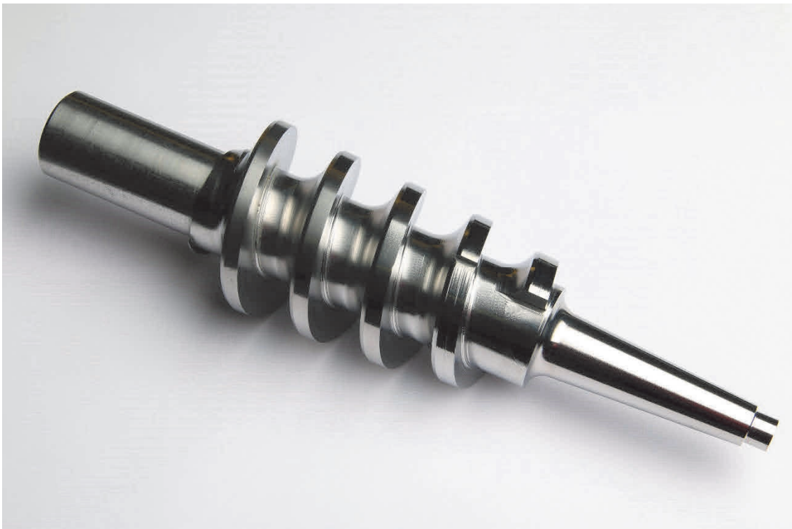
Figure 2 The milling screw prepared for laser cladding
