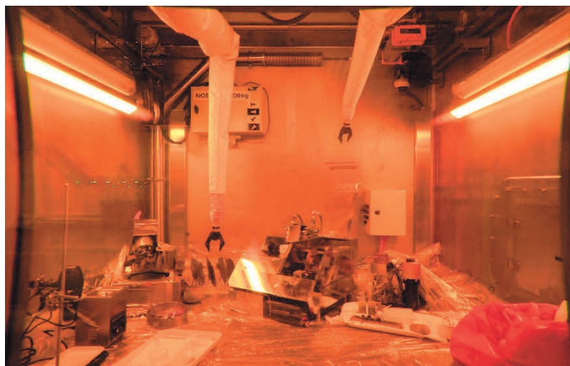
Figure 3 Metallographic hot cell prepared for operation with active samples
