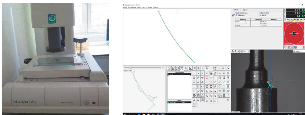
Figure 4 Vertex 251 HM optical precise measurement device
