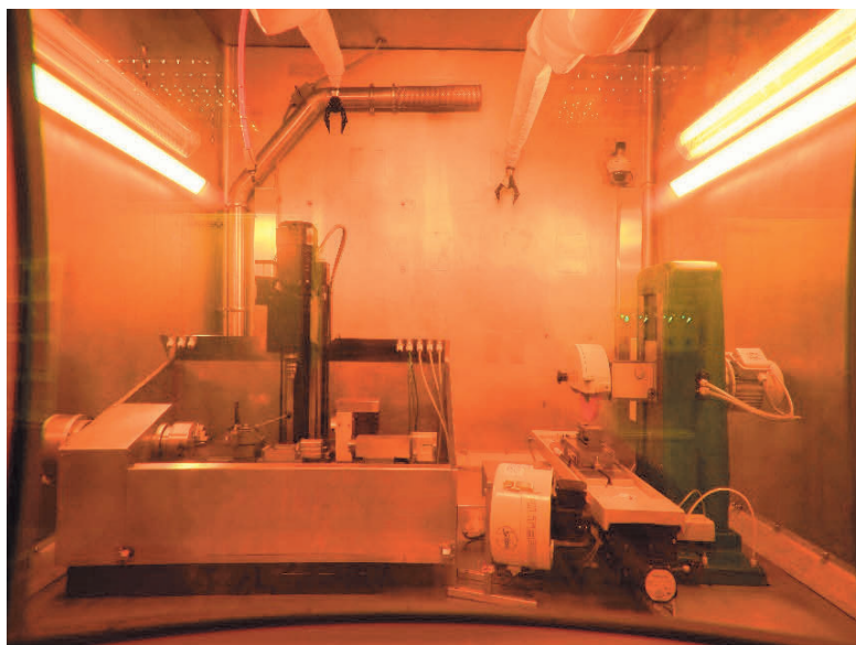
Figure 2 Mikronex CNC machining center inside the CVR hot cell
