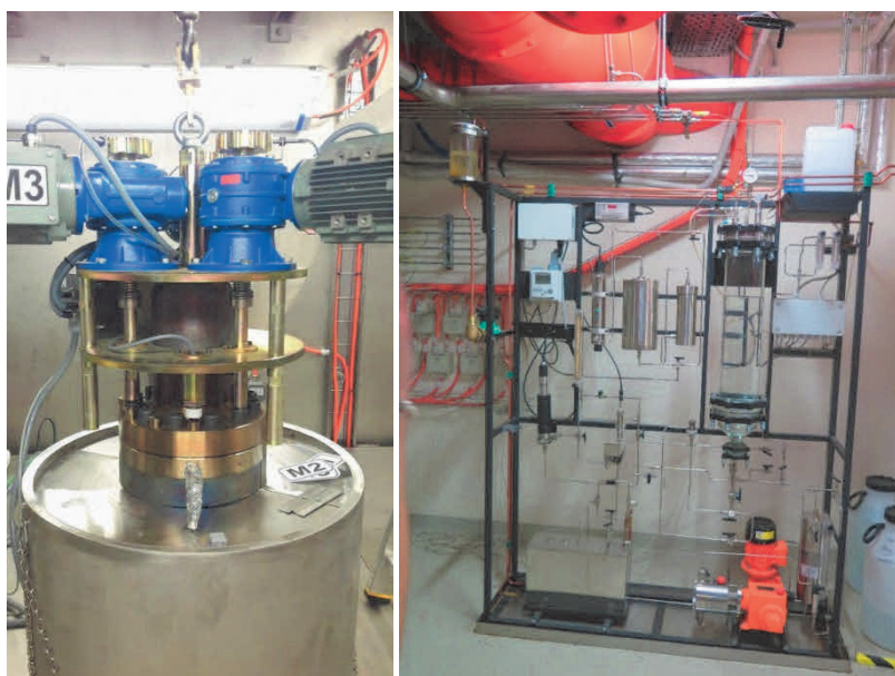
Figure 5 Images of the autoclave body with a tightening system (left) and a water loop (right)
