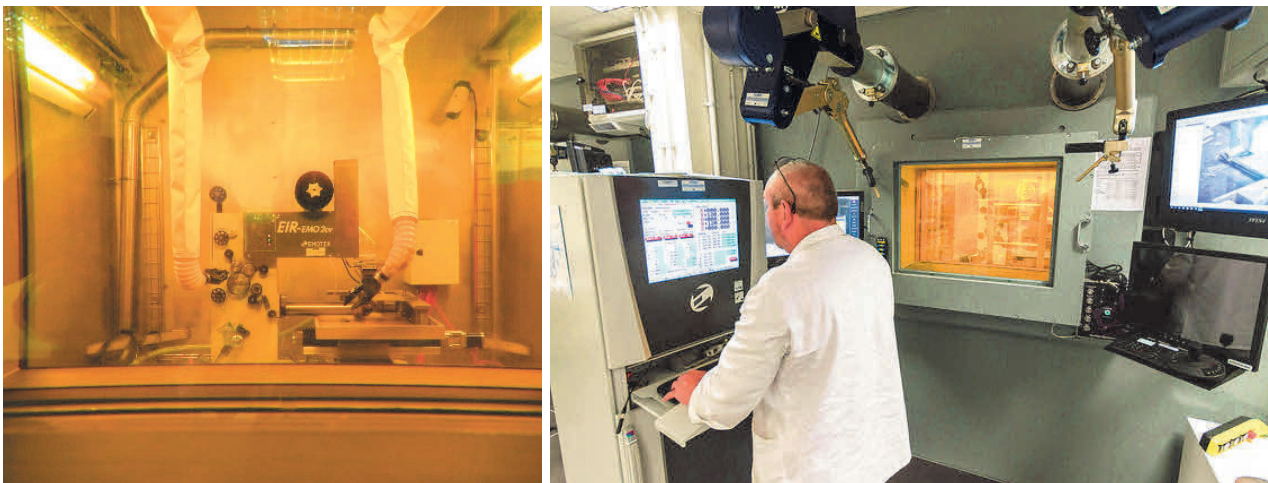
Figure 1 EDM machine inside the CVR hot cells for cutting and machining of irradiated samples (left) and the distanced operation of the machine (right)
