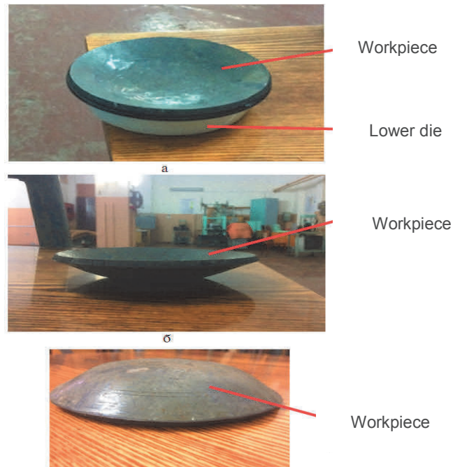
Figure 3 The obtained experimental sample: a) the detail and the bottom base (matrix) of the package in the assembly; b) general view of the part; c) the shape of the lower surface of the part
