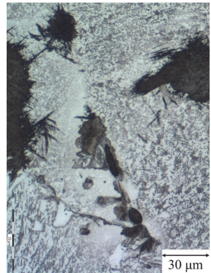
Figure 4 A bainite-perlitic structure of alloy B
