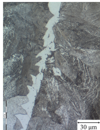
Figure 2 A perlitic structure of alloy A
