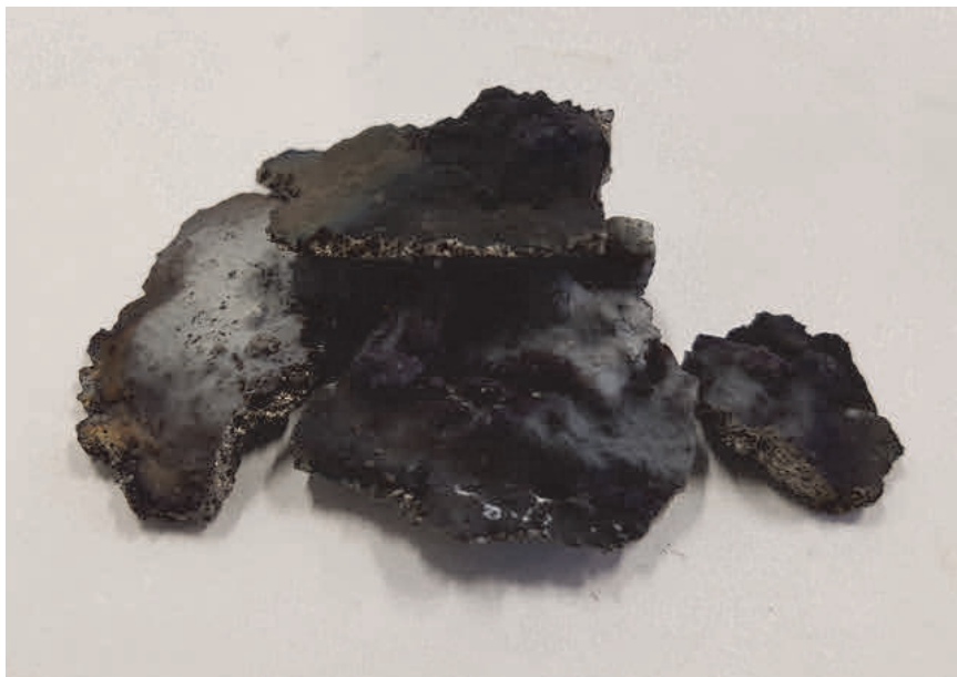
Figure 1 The example of the product of self-propagating high temperature synthesis of Ti-Si intermetallic phase
