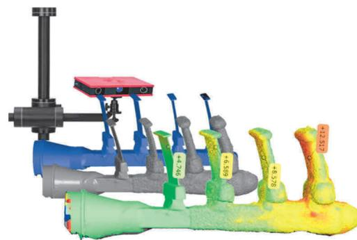
**Figure 2** Diagram of digitizing the ceramic form using the GOM ATOS CORE system
