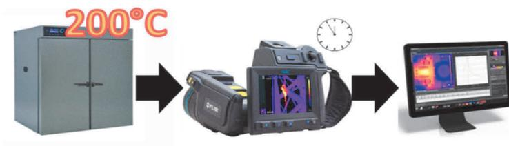
**Figure 3** Diagram of thermovision tests
