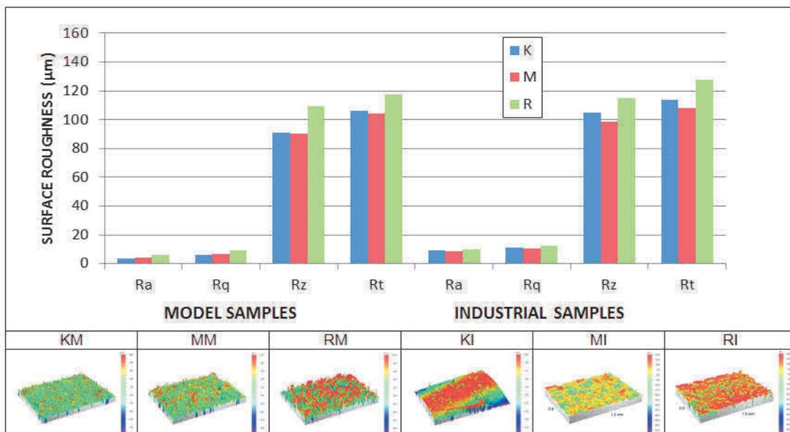
**Figure 4** Surface roughness of the first model coat after heat treatment at 900 °C
