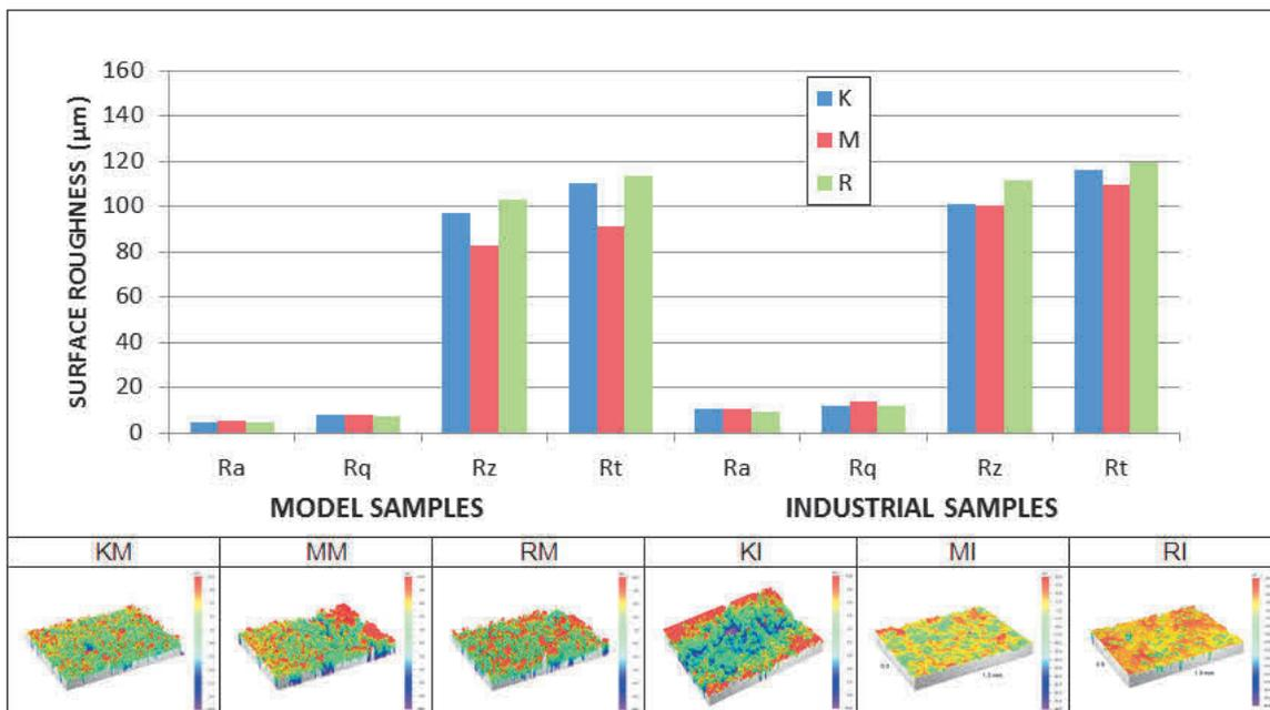
**Figure 3** Surface roughness of the first model coat after heat treatment at 850 °C
