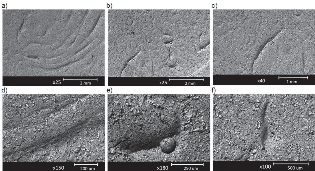
**Figure 9** Structure of surface of the model layer after heat treatment at 950 °C for materials K (a, d), M (b, e), R (c, f)
