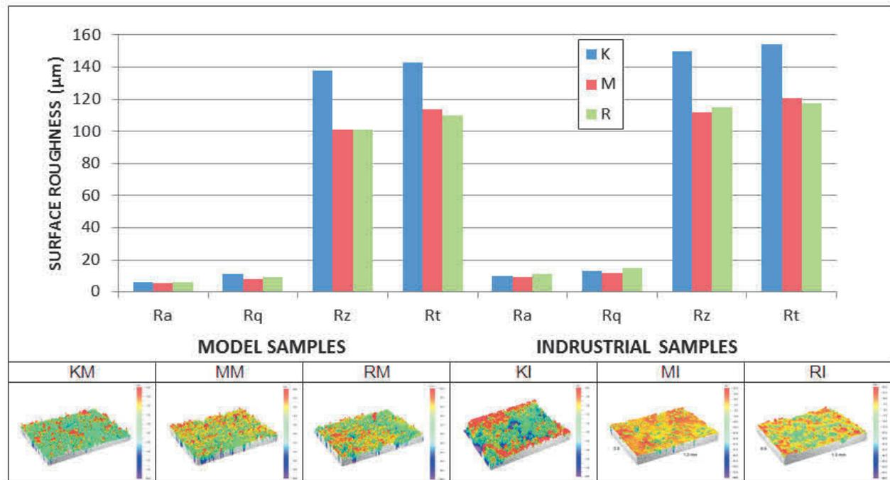
Figure 5 Surface roughness of the first model coat after heat treatment at 950 °C
