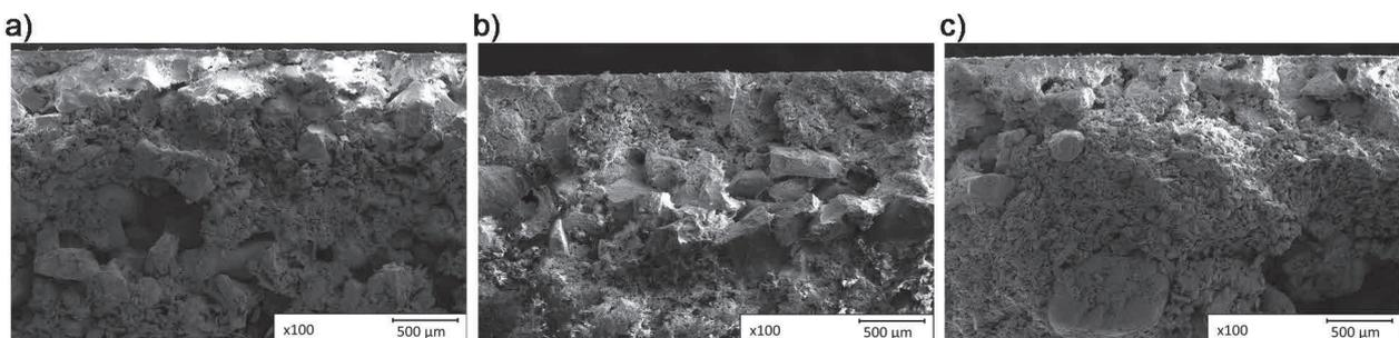
Figure 6 Structure of moulds made of material K (a), M (b), R (c) after heat treatment at 850 °C
