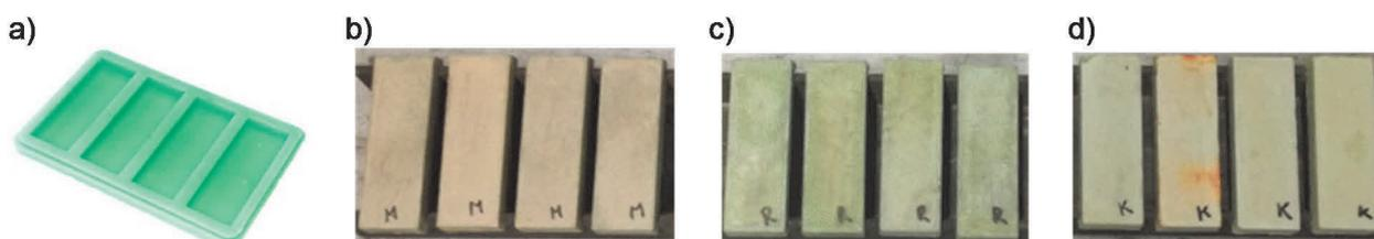
**Figure 1** Wax die (a) and model ceramic samples: M (b), R (c), K (d)
