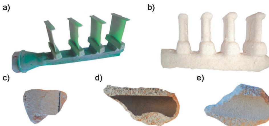
**Figure 2** Wax model set (a), ceramic mould (b) and industrial ceramic samples K (c), M (d), R (e)
