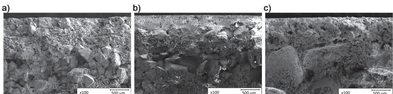
Figure 7 Structure of moulds made of material K (a), M (b), R (c) after heat treatment at 900 °C
