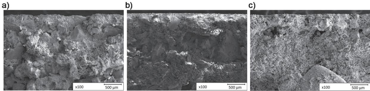
**Figure 8** Structure of moulds made of material K (a), M (b), R (c) after heat treatment at 950 °C
