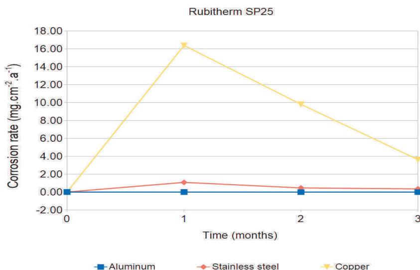
Figure 3 The dependence of corrosion rate CR (%) on exposure time for Rubitherm SP25
