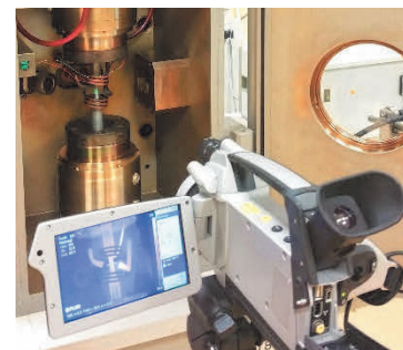
Figure 4 An AlZn5.5MgCu aluminum alloy specimen in the chamber of the STD 812 torsion plastometer
