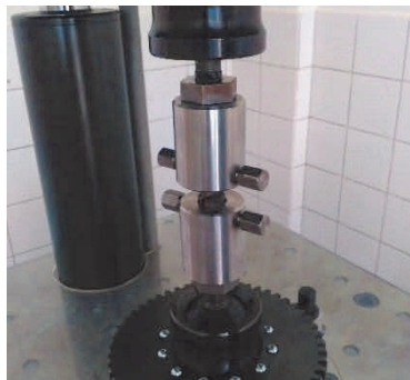
Figure 4 Clamps for miniature test specimen
