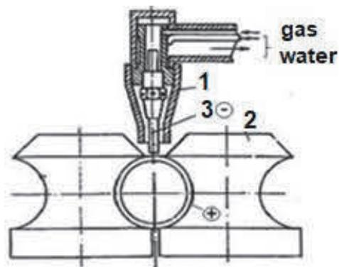
**Figure 2** Seam tubes welding by TIG method
