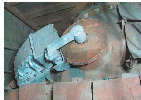
Figure 3 Scheme of the plug-type stopper principle and its detail on the oxygen converter tap hole [4]
