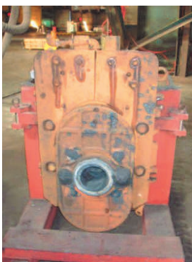
Figure 4 View of the slide gate stopper prepared for instalation and scheme of its mounting on the oxygen converter tap hole [6]
